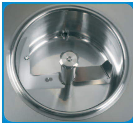
• Cylinder and beater detailed view
